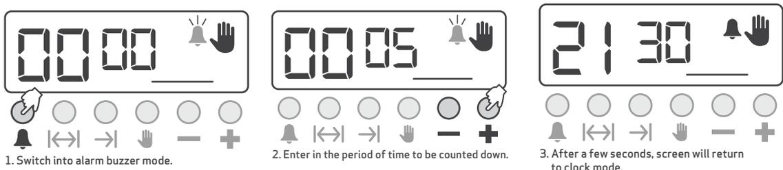
**Note:** Once programmed, the remaining time can be seen by pressing the 🔔 button once.
