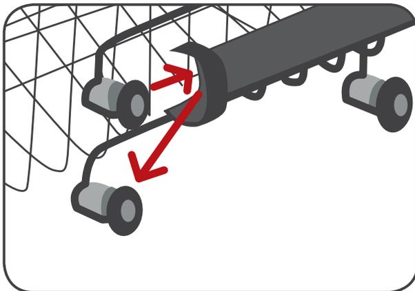
In order to change the height, remove the basket by shifting the clip at the end of the rail to the side.
