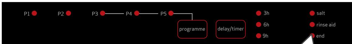
The end of programme indicator turns on when a programme is complete. Your machine will also sound a buzzer five times.
