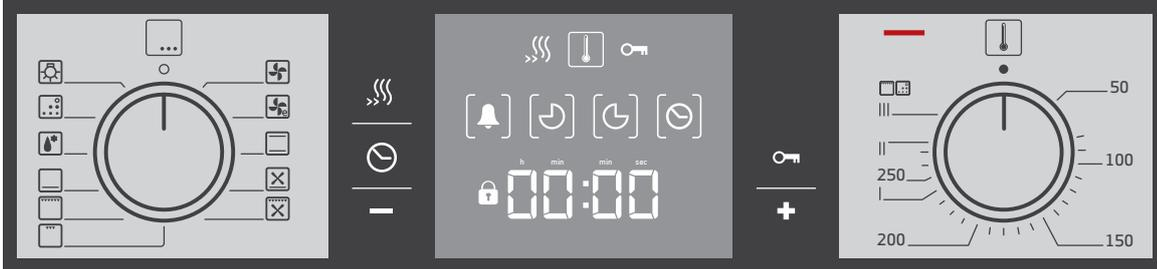
The control knobs are retractable. To lock it in or out, press the control knob in the off position.
