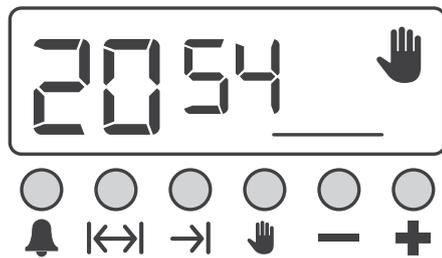
This Montpellier oven has a programmable timer. This enables you to programme the cooking of your food to be ready at a desired time. You can just programme the oven to come on at the time you require and at the correct temperature. It can also be used as a minute minder which has an end time audible alarm.
