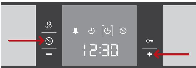
After a few seconds the oven adopts the settings and switches to standby position. The time at which the dish will be ready is shown in the display and the ☺ symbol is in brackets. The 🔔 and ☹ symbols go out. When the oven starts, you can see the cooking time counting down in the display and the ⌚ symbol is in brackets. The ☺ symbol goes out.
