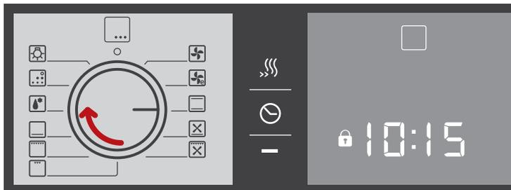
2. Set the temperature or grill setting using the temperature selector
